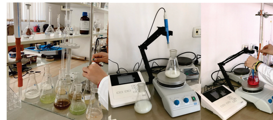
Figure 14: Total acidity determined with potentiometric method
