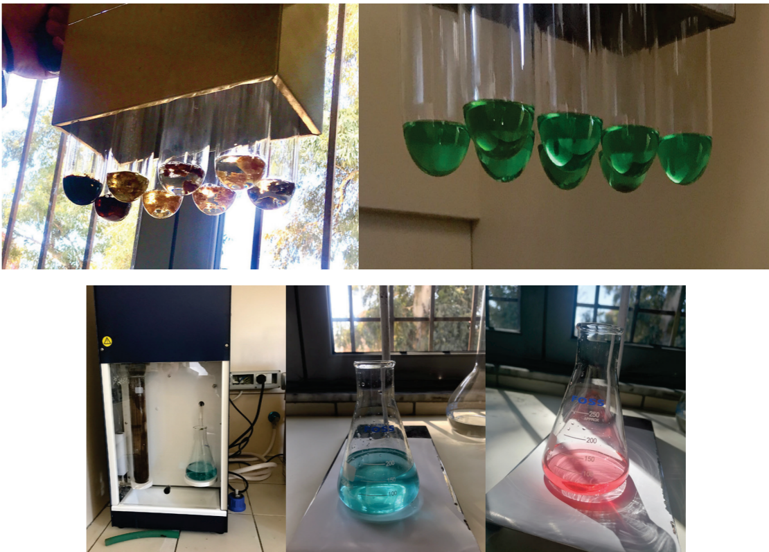
Figure 10: Total protein determined by Kjeldahl method
